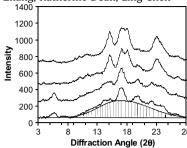
X-ray diffraction patterns of cornstarches with different amylose contents (from top to bottom: waxy, normal corn, G50, and G80). The portion of the dashed indicates the amorphous area.
